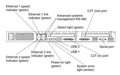
**Ethernet 1 speed indicator:** This green LED lights when the speed of the Ethernet LAN that is connected to Ethernet port 1 is 100 Mbps.
