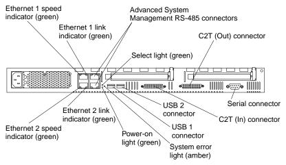
The ASM ports on the back of the server are referred to in this book as RS-485 (A) and RS-485 (B).
