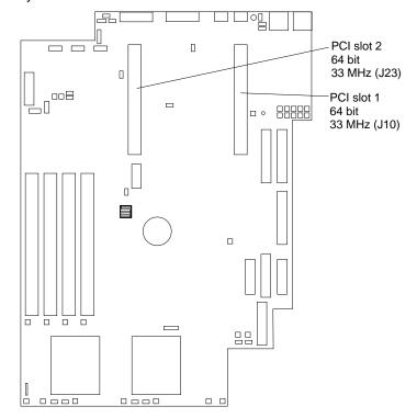
The following illustration shows the location of the 33 MHz PCI expansion slots on the system board.
