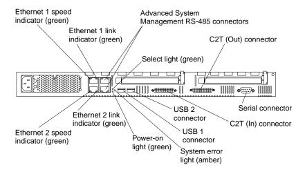
**Ethernet 1 speed indicator:** This green LED lights when the speed of the Ethernet LAN that is connected to Ethernet port 1 is 100 Mbps.
