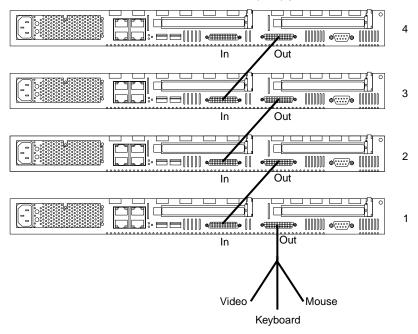
**Note:** Server 1 (usually the server at the bottom of the rack) is the server to which you connect the device breakout cable.
