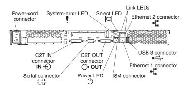
Power-cord connector: Connect the power cord to this connector.
