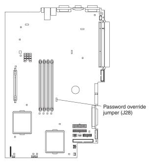
Complete the following steps to change the position of the password-override jumper:
