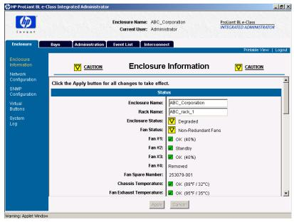
Figure 6-7: Viewing the Web-based user interface of the Integrated Administrator during a fan failure
