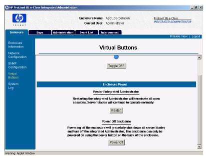
Figure 3-10: Virtual Buttons screen (Enclosure Power area)
