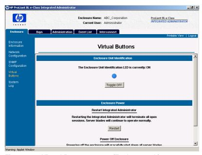
Figure 3-9: Virtual Buttons screen (Enclosure tab)
