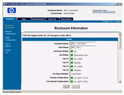
Figure 3-5: Enclosure Information screen (status area, 1 of 6, shown)
