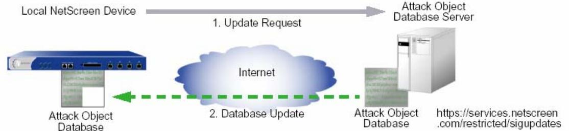
The update process entails connecting to the Juniper Attack Object Database Server, which will be updated regularly with new attacks and updates to preexisting attacks. Emergency updates will also be provided to protect against key attacks as necessary. Customers must have a software subscription and subscribe to the Target Attack Update Service to receive these new attack protection enhancements.
